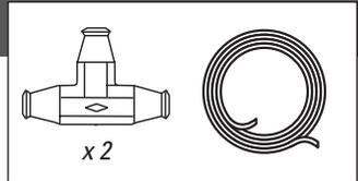
**1** Route the air line tube from 1/8 NPT push-to-connect straight fitting on the top of the air compressor to the first 1/4" push-to-connect tee.
