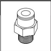
**1** Thread 3055 air fitting into air spring combo stud.
