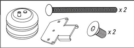
**1** Install 3502 carriage bolts through square holes in 5945 bracket.
