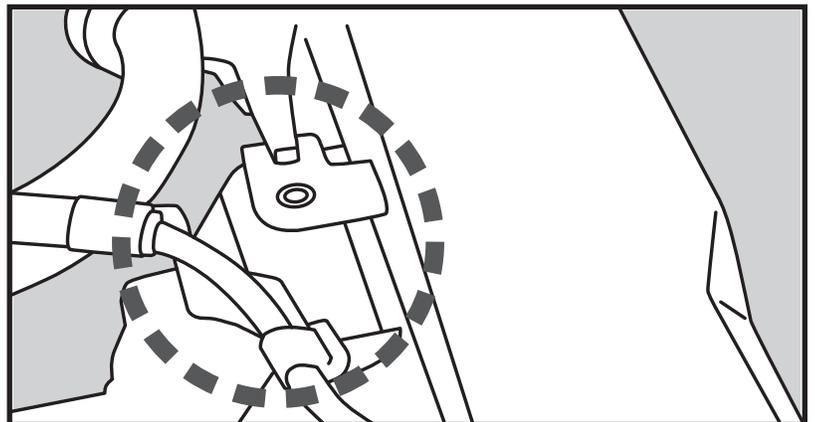
LOOSELY ATTACH LOWER BRACKET TO AIR SPRING BOTTOM
