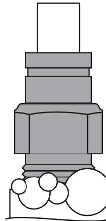
Tighten Air Fitting one turn or until leak stops.
