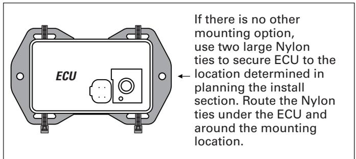
If there is no other mounting option, use two large Nylon ties to secure ECU to the location determined in planning the install section. Route the Nylon ties under the ECU and around the mounting location.
