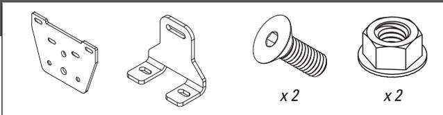
**1** Attach 5944 to 5943 using 3514 bolt and 3022 flange nuts in holes shown.
