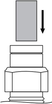
**2** Push air line tube into air fitting as far as possible.
