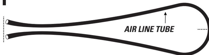
**2** Find center of air line tube, make a square cut with tube cutter or sharp utility knife.
