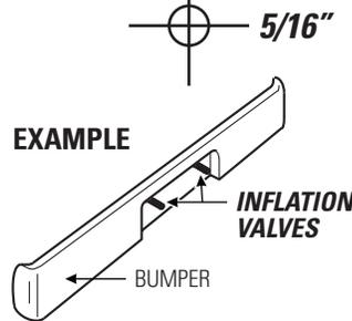
**3** Install inflation valve assembly as shown.
