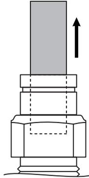
**4** To remove, push down collar and gently pull air line tube away.
